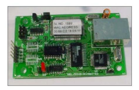
The EAD is the most cost effective Single port Serial-Ethernet communication device. The EAD supports RS232 serial communication allowing virtually any asynchronous serial device to be accessed over a network. Some models do Support RS 485 and RS422 as add-on feature. As for the Internet connectivity, the EAD supports open network protocols such as TCP/IP allowing Serial Devices to be accessed over broadband network or conventional LAN (Local Area Network) environment.
