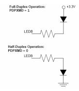
• Upon system Reset, the ENC28J60 will detect how the LED is connected and begin driving the LED to the default state
